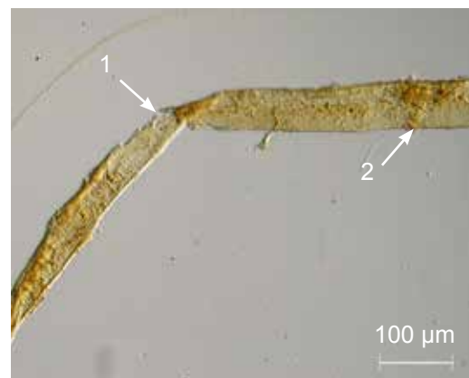
Fig. 6 Fibre from fore-edge: complete fibre with no flexibility (1) and many residues on the surface (2), possibly damaged and dried out by heat (see Fig. 3) (HNA 53, dated 1340)
