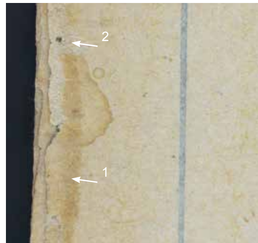
Fig. 9 Edge of folio, brittle paper, caused by iron content; glue of paper-sizing was reactivated by entering water stopped through the swelling effect (small water stain along border [1]); after separation from next folio (loss of paper surface within water stain [2]) (HNA 18, 17 th century)
