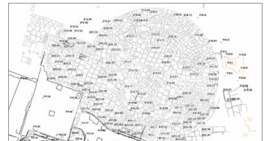
Fig. 385 Documentation: combination of drawing and total station measurement
