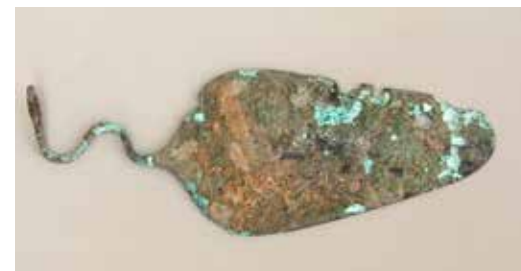
Fig. 3 Example of aggressive corrosion that has partly destroyed the object (HNM 010.05.07c, cat. no. Pr13)
